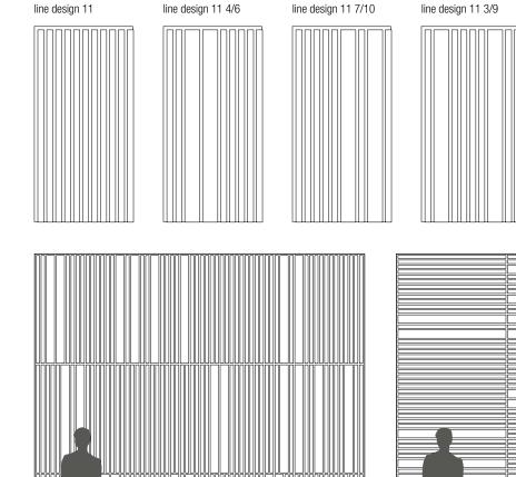
Troldtekt line design installed vertically
