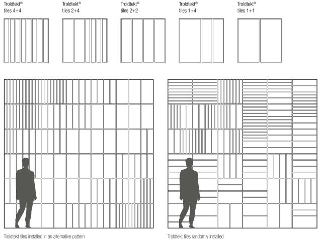
Troldtekt tiles installed in an alternative pattern
