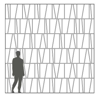
Troldtekt tilt line installed horizontally
