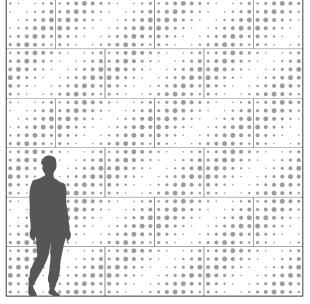
Troldtekt dots installed in horizontal stretcher bond
