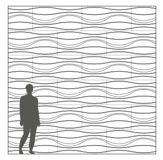
Troldtekt curves installed in horizontal stretcher bond
