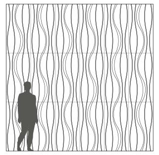
Troldtekt curves installed in vertical stack bond
